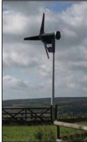
Figure 3: 6 kW turbine on a 9m mast (5.5 m diameter). Townfield Head Farm, Stannington
