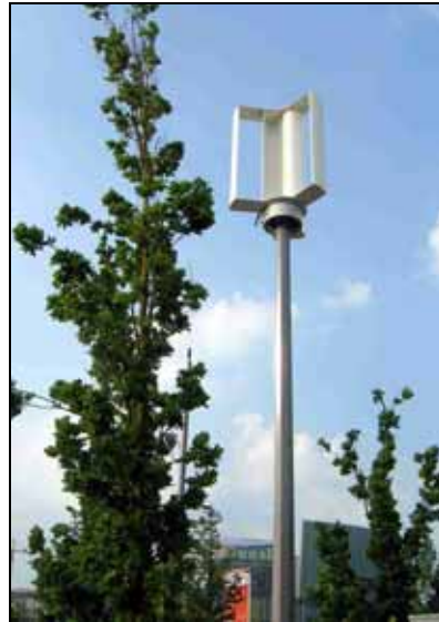
Figure 2: Vertical Axis Wind Turbine (1 kW) TASSA GmbH
