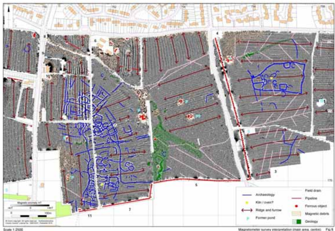
Fig 4 The anomalies in blue shown on this extract from the geophysical survey indicate the extent of Iron Age and, probably Roman period settlement in the central western section of the development area.
