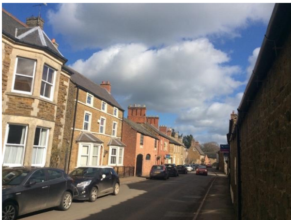
Mix of ironstone walls, red brick walls, dressed stone mullions, bays, slate roofs and string courses (High Street, Somerby).
